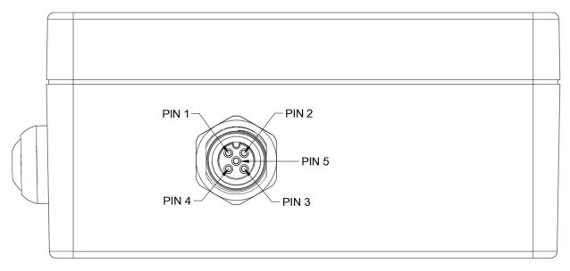
\*See "SDI-12 / MODBUS Sensor M12-5 Connector Wiring Reference" for appropriate sensor wiring.
