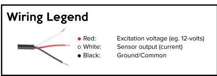
Note that in unusual circumstances (for example if the sensor is immersed completely in water) the output current can exceed 20mA. If this could be harmful to connected equipment, appropriate protective measures should be taken.
